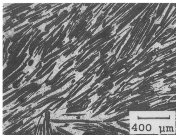
Figure 14 Photomicrograph of a graphite flake particulate composite.
